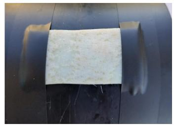
Figure 3. Porcine skin specimen constrained to backing surface
