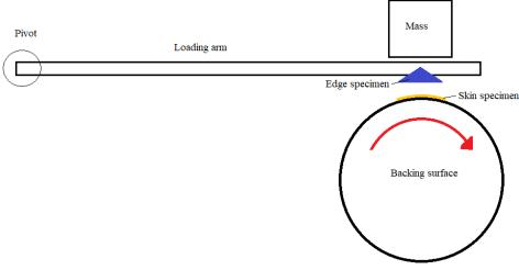
Figure 2. Diagram of test setup
