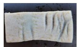
Figure 8. Damage patterns from plastic edge
