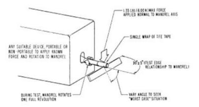
Figure 1. Principle of sharp edge test for CFR 1500.49
