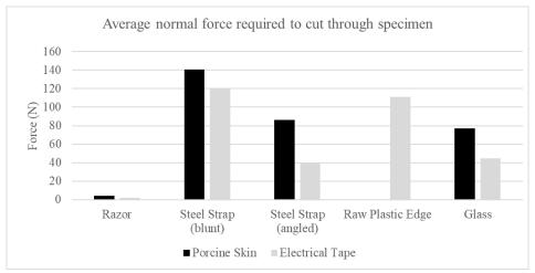
Figure 6. Force required to cut through specimen
