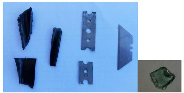
Figure 4. Edge specimens. ABS plastic with raw edge (left), steel hanger strap, razor blade, and broken glass.
